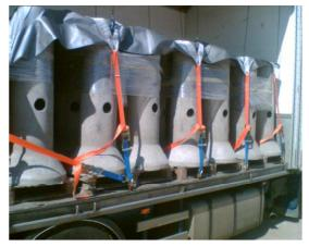
Surface pressure caused by tensioning is divided over entire surface and will therefore not damage the load. Sensitive load and soft packages cause no problem. Also, when high acceleration forces are applied, the load will not be damaged.
