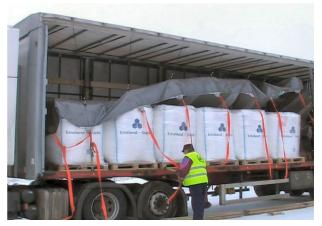
the vehicle. The length can also be divided to several shorter tarpaulins and versions to cover the end of the load are also possible. Blocking the end of load from moving forward is very effective method to secure the load. When
