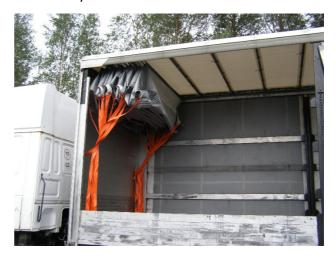
not in use FIX Road® can easily be stored against one end of the vehicle. Space requirement is only 60cm.
