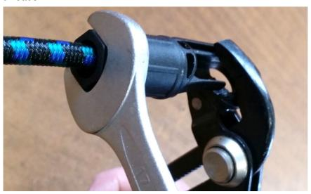
When hand force is not enough, take a steady grip of the hook with pliers and turn the nut with wrench until the nut is completely on place.
