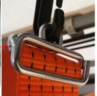
On the hook side the strap is thread through FIX Slide like in the pictures. Do not thread the strap any other way as then the adjustment is more difficult and tension in the strap when tightened will deform FIX Slide.
