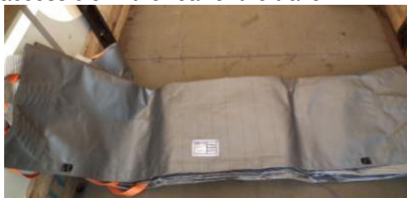
Figure 16. Spread out the Fix fabric with the tag to the rear of the trailer.
