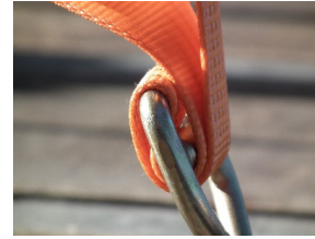
Figure 24. & 25. Adjustable hook and how the strap is routed
