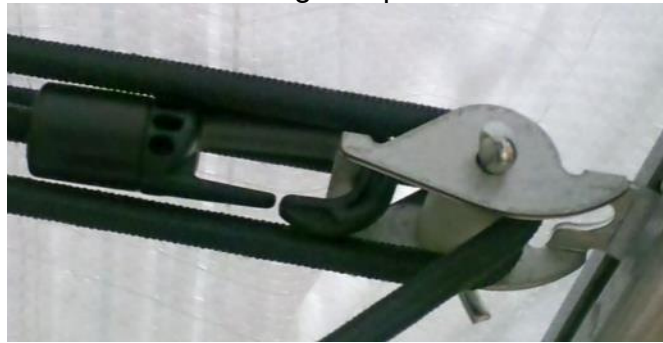
Picture 14. Correct position of roller carriage and bungees.
