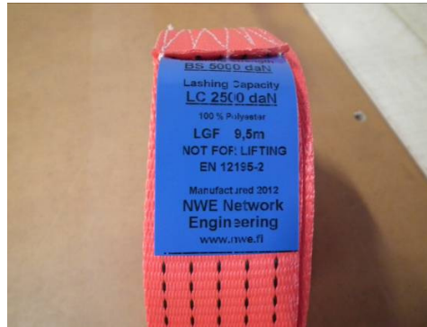
Figure 17 & 18. Tag for the type code tells (from top down) the size and model of the cover, production month and year, serial number, DEKRA approval number, number of straps and strap length . Tag for strap tells breaking strength BS, lashing capacity LC, material, length, applied standard and manufacturer.
