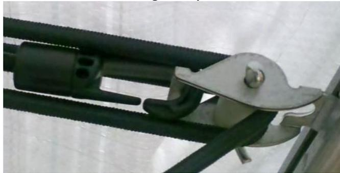
Picture 14. Correct position of roller carriage and bungees.
