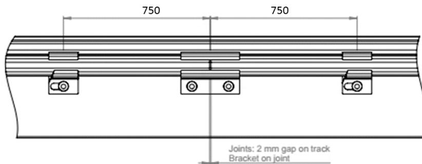
Drawing 11. Wall mounting brackets and a wider joint bracket over the track joint.
