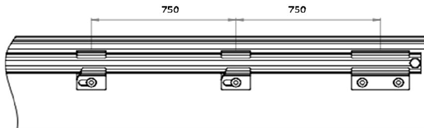
Drawing 15. Locking bolt and last wall bracket mounted.
