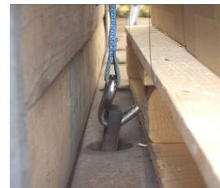
When unloading the cargo, and loosening the ratchet, the bungees will pull the strap up to the roof again and it can be sliding out of the way.
