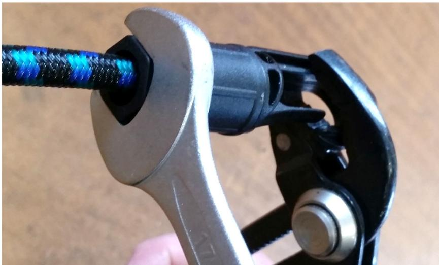
When hand force is not enough, take a steady grip of the hook with pliers and turn the nut with wrench until the nut is completely on place.
