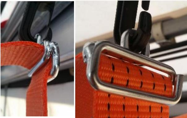
On the hook side the strap is thread through FIX Slide like in the pictures. Do not thread the strap any other way as then the adjustment is more difficult and tension in the strap when tightened will deform FIX Slide.
