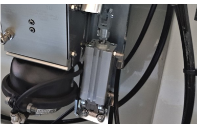
Locking cylinder FIX Truck-safe Locking cylinder for automatic tensioner.
