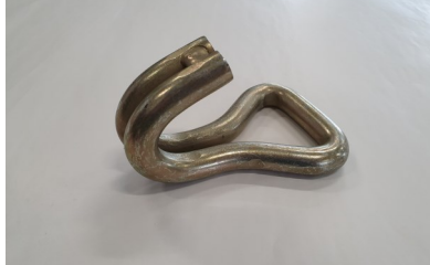
Hook Strap hook 50mm D32mm LC 25 kN
