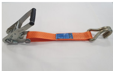
FIX ratchet 0,4 with d32mm J hook 0.4m Ratchet tensioner ends with wire J hook d32mm 50mm SHF 50 daN, STF 300 daN LC 2500 daN
